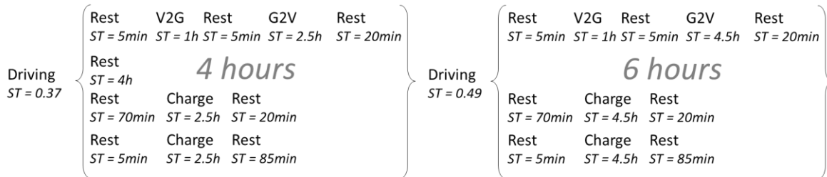
Figure 16: Test duration and step limit for actual experiment.
