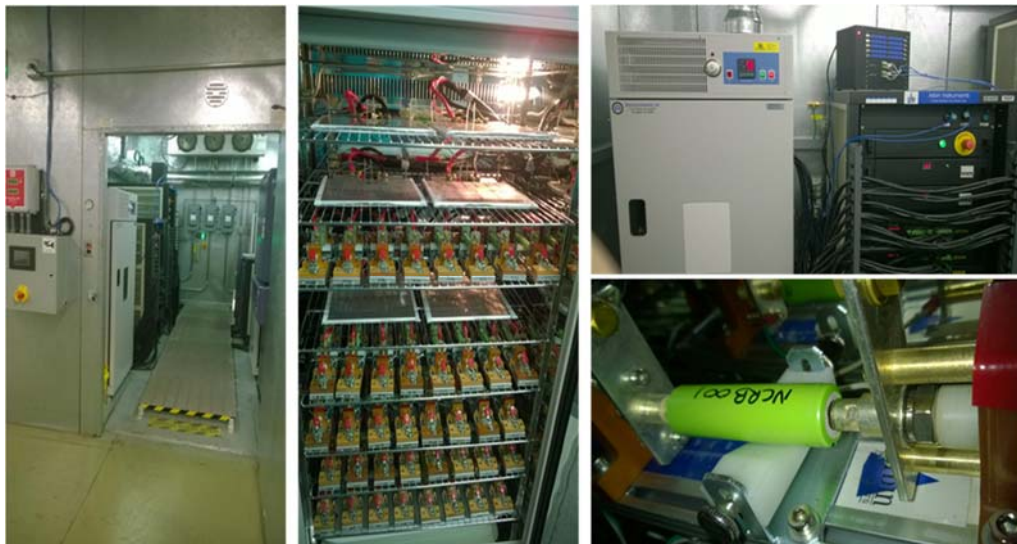
Figure 1 - Battery testing laboratory entrance, inside temperature chamber, temperature chamber and battery tester & a commercial “18650” Li-ion cell used for the EVTC project in battery holder. (Photos: Dr. Arnaud Devie, HNEI)
