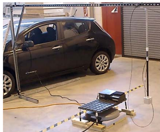
Figure 2 - Automated Test Stand w/ Stepper Motor Actuator (Photo: FSEC)
