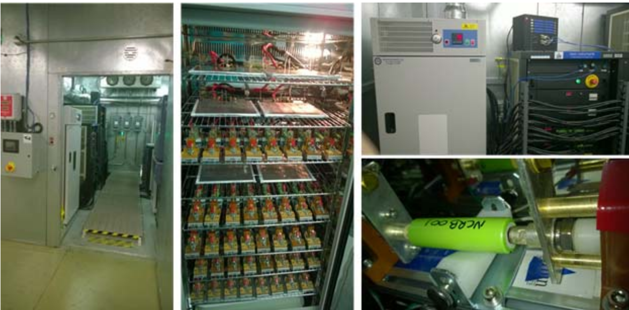
Battery testing laboratory entrance, inside the temperature chamber, temperature chamber and battery tester & a commercial 18650 Li-ion cell used for the UTC project in a battery holder. (Photos: Dr. Arnaud Devie, HNEI)
